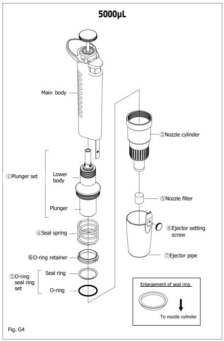
Circled Numbers in (Fig. G4) corresponds to Parts Numbers in the replacement parts list.
