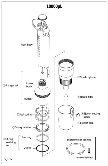
Circled Numbers in (Fig. G5) corresponds to Parts Numbers in the replacement parts list.
