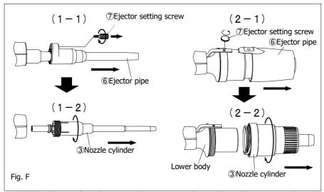
Circled Numbers in (Fig. F) corresponds to Parts Numbers in the replacement parts list.
