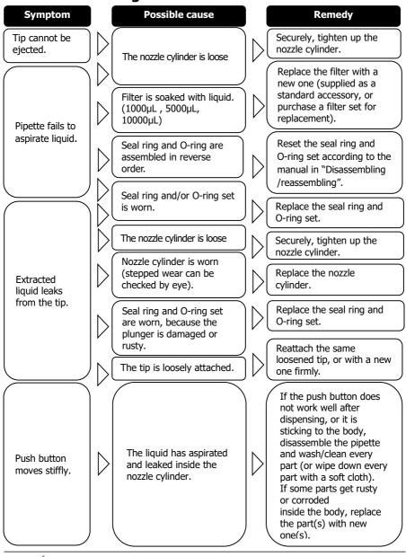
When the pipette cannot be fixed after examining and conducting the above mentioned procedure, immediately stop using the pipette and ask us or our agent to repair it.
