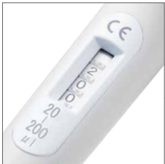
Enlarged and easy to read counter display for volume setting.
